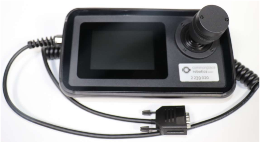
Figure 4.8: Operating Panel with touch screen and 3-axis joystick.
